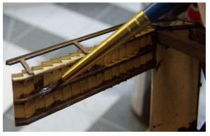
(Below) When adding the corner trim, the deck corner end trim needs to be cut as shown for the deck to fit flush against the building
