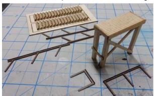
The below right image show all the railing added and the steps glued to the deck.
