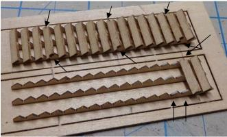
Above image is the deck bottom and top section to be glued together. The right image shows the 3 legs, bracing and deck side boards installed. Below shows the top section added to the railing.
